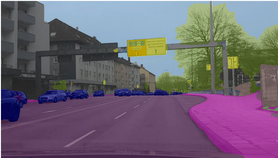
Figure 66: Example of a so-called semantic segmentation, calculated by a deep neural network. For each image pixel a class membership is estimated, by an assignment of classes to colors such a segmentation image is created.
