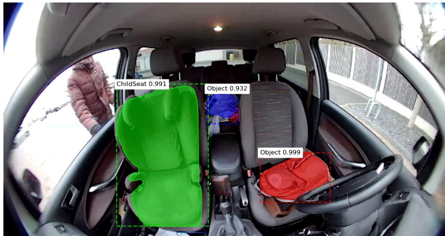
Figure 68: Example of instance segmentation in the interior of a car. First, objects are localized and outlined by rectangles. Then the instance is segmented within the rectangle.
